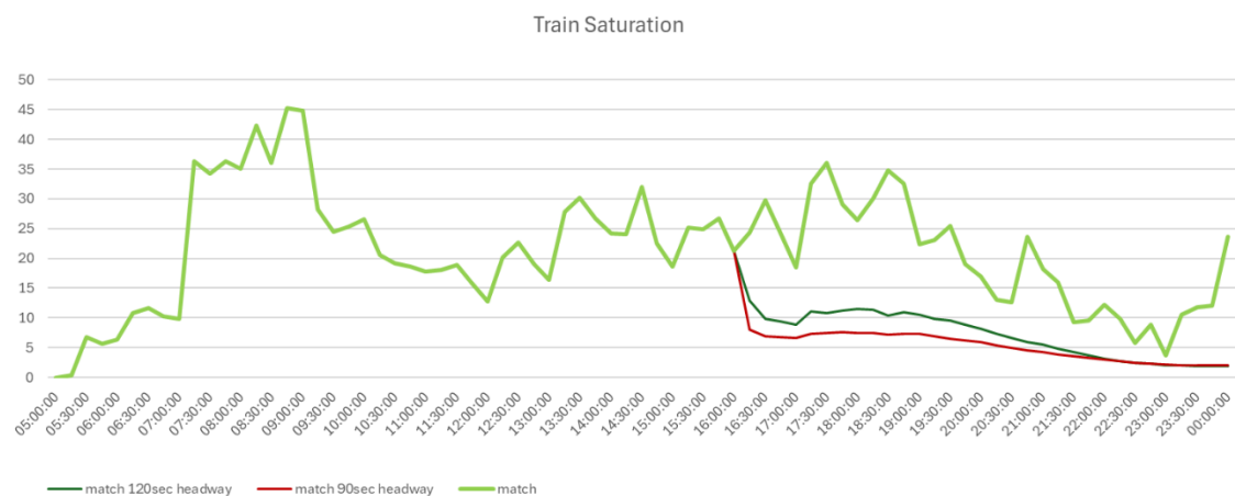
Figure 6: Train saturation levels between current and fully automated operations (Match Day)
